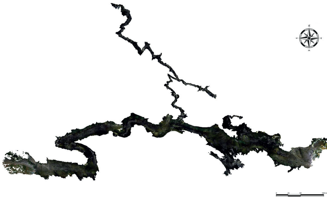
Figure 4: The laser scan survey obtained merging all point clouds.
