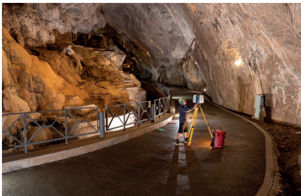
Figure 5: The Leica P40 laserscanner along the in-cave road (Photo Vittorio Crobu).
