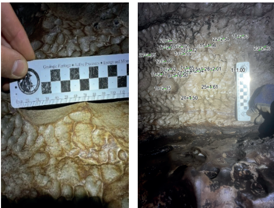
Figure 2: Left shows a physical measurement with a scale. Right shows a measurement taken of a scallop remotely. Note “1=1.00” for defining scale. Source: author.
