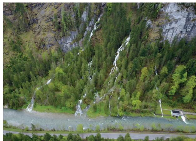
Figure 1: Drone photo looking diagonally down towards the south at the Kläffer Springs, taken during the snowmelt on 9th May 2017 with a total discharge of 14 m 3 /s. The water for the city of Vienna is collected underground in a tunnel near the building in the bottom right corner. In winter or during long periods of low discharge, (almost) none of these surface waters are present. Width of the river in the foreground 0.25 km.
