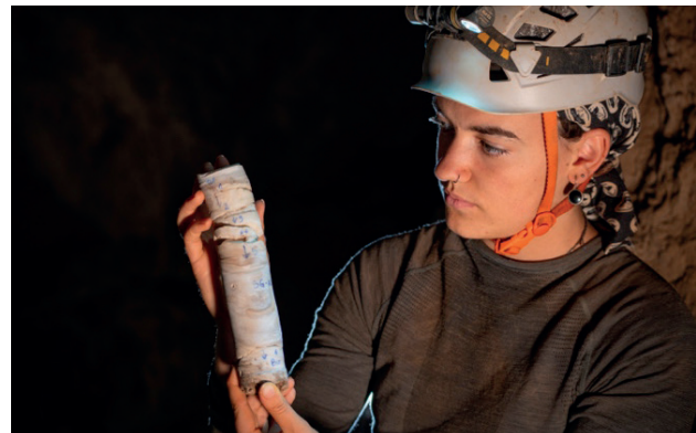
Figure 3: One of the speleothem samples taken through handheld battery-powered drilling (Photo Vittorio Crobu).
